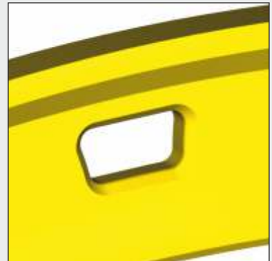
Deckeldurchbruch gefräst Turned cap with milled window
